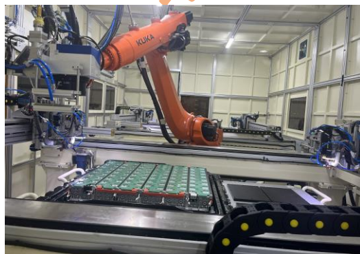
试制电池包汇流排激光焊接
